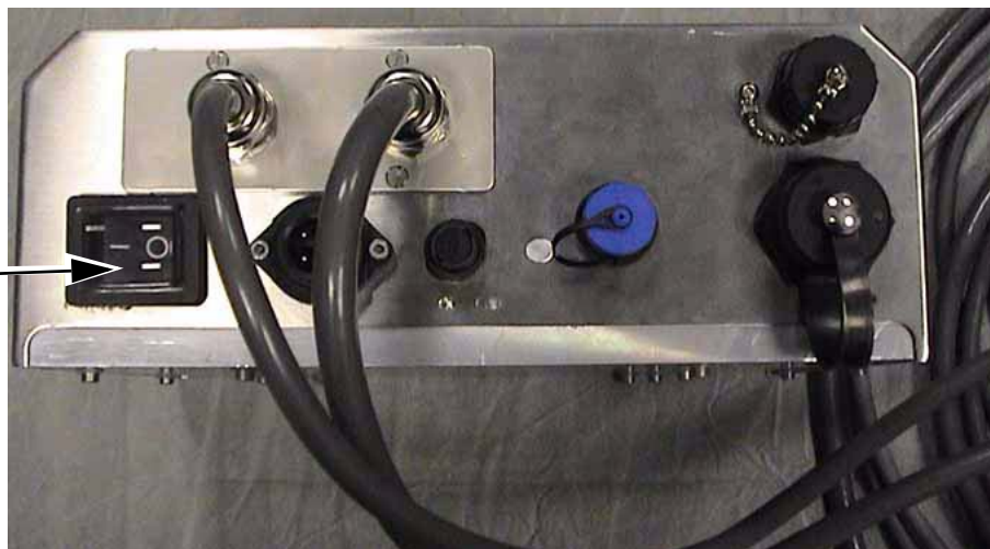
Figure 3-3: IP Printer Power Switch
