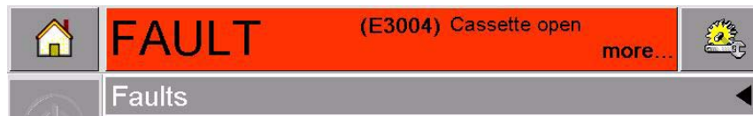
Figure 5-5: Cassette Open Fault
